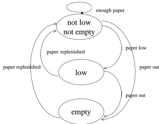
The threshold status of the retract bin may change according to the following state transition diagram:
